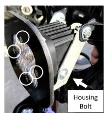
Using the 7/16" wrench and socket wrench, tighten the ¼" bolt into the washer, plastic bracket, steel bracket, washer, and nylon locking nut. Repeat for the adjacent fastener.
